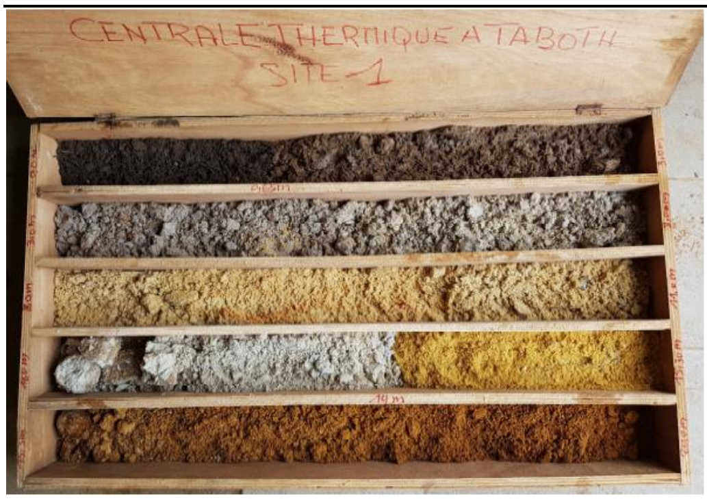
Figure 6.4 Coupe de sol, carottage SC1
